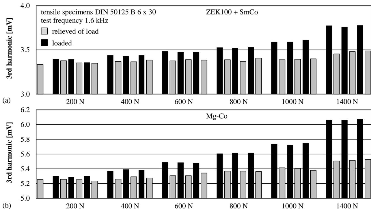
**Figure 2.** Measured amplitudes of the 3<sup>rd</sup> harmonic depending on the applied load; alloy ZEK100 + SmCo (a), alloy Mg-Co (b).
