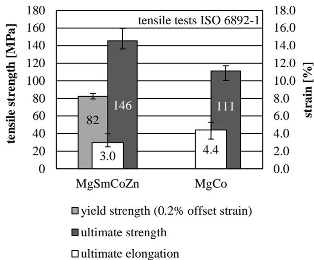
**Figure 3.** Mechanical properties of the alloy ZEK100 + Sm and the binary Mg-Co alloy in as-cast condition (n = 6).
