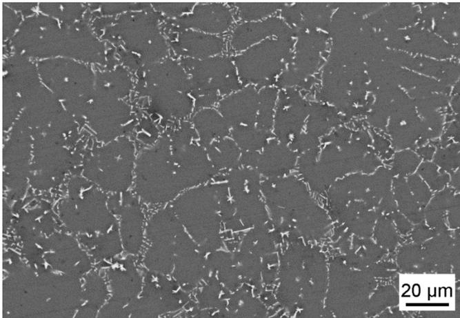
**Figure 1.** SEM image (RBSD mode) of the microstructure of the binary Mg-Co alloy.
