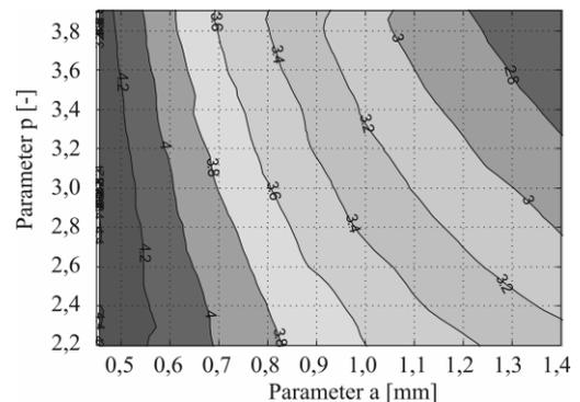
**Figure 7.** Influence of  $a$  and  $p$  on strains sensitivity.
