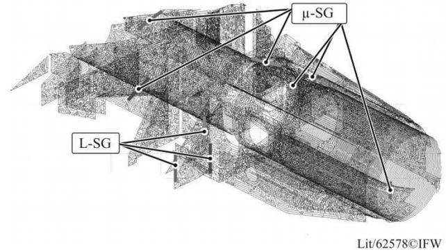
**Figure 3.** Optimized sensor positions on the Z-slide.
