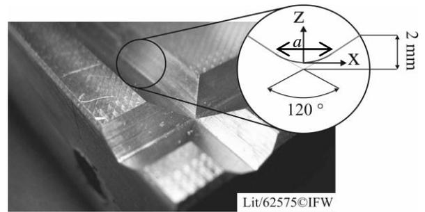
**Figure 6.** Notch geometry and manufactured sample notches.
