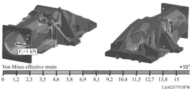
**Figure 2.** Simulation results for sensor amplitude estimation.
