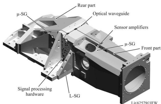
**Figure 1.** Concept for the sensing Z-slide with light fibre communication and micro strain sensors.
