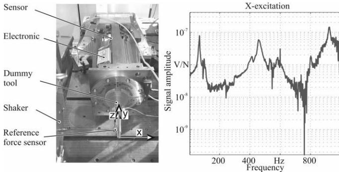
**Figure 5.** Test setup and frequency response of strain sensor 1 in sensing Z-slide.
