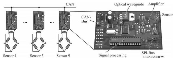
**Figure 4.** Signal processing and communication of the sensory Z-slide.
