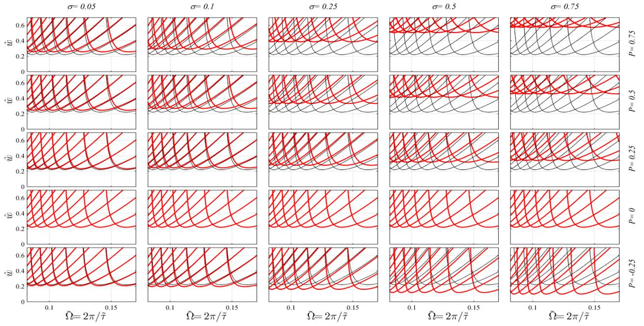
**Figure 3.** Stability boundaries of the turning process (red thick lines: control with distributed delay, black thin line: no control).
