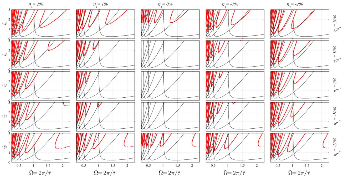
**Figure 2.** Stability boundaries of the turning process (red thick lines: control with point delay, black thin line: no control).
