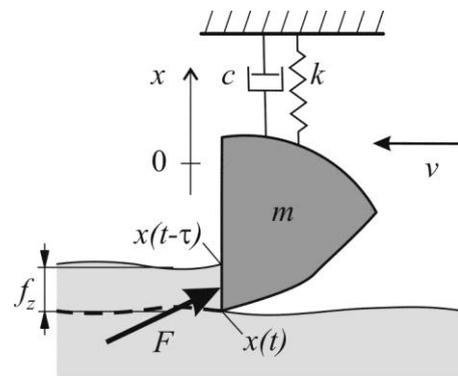
Figure 1. Mechanical model of the orthogonal turning.
