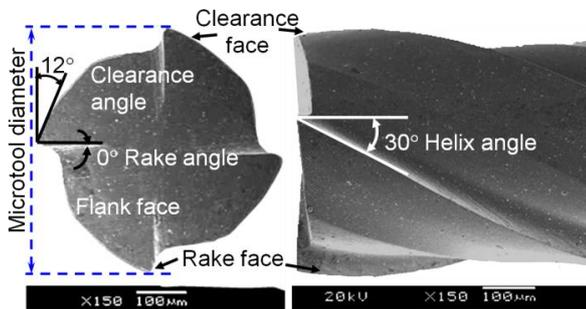
**Figure 1.** SEM micrograph of a new micro end mill.
