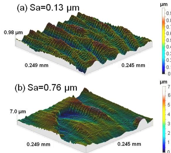
**Figure 3.** 3D topography plots of surfaces produced using; (a) new, (b) worn tools (2600 mm cut length).
