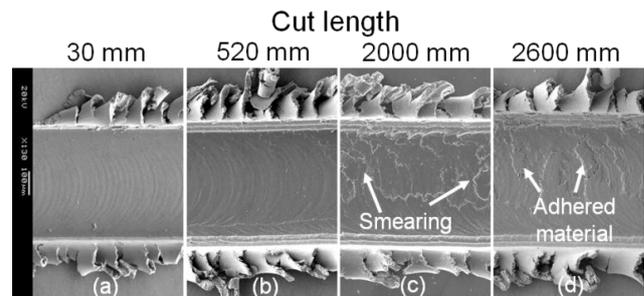
**Figure 2.** Typical slot surface roughness progression.
