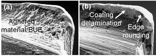
Figure 4. Condition of tools used in; (a) Test 7, (b) Test 8.
