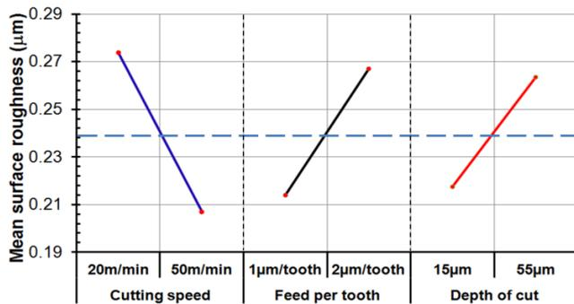
Figure 5. Main effects plot for mean surface roughness.
