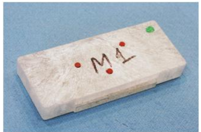
Figure 5. Plastic mounting with three TGs fixed in it using resin plugs.
