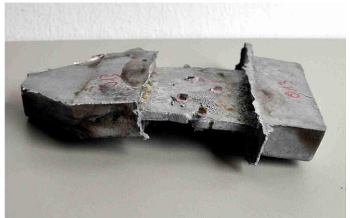
Figure 8. Deformation of an aluminum casting part.
