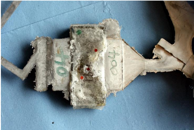
Figure 6. Mounting with three TG embedded in cast aluminium.
